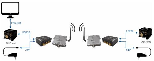
Microhard + amplifier radios and Autopilot 1x operation
