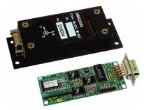
**Magnetometer Honeywell HMR2300**
