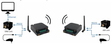
DTC radios and Autopilot 1x operation
